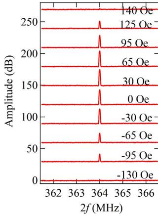
Fig. 5. Voltage spectra under the microwave magnetic field with the frequency of 182 MHz for various static in-plane magnetic fields.
