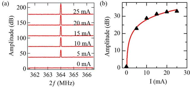
Fig. 4. (a) Voltage spectra under the microwave magnetic field with the frequency of 182 MHz for various dc current in the absence of the magnetic field. (b) Current dependence of the amplitude of the resonant peak of the second-harmonic signal. Solid line: logarithmic curve fitted to the experimental data.
