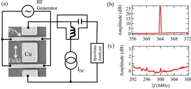
Fig. 2. (a) Circuit diagram used for the second-harmonic signal measurement together with the scanning electron microscopy image of a part of the fabricated device. (b) Representative voltage spectrum under the microwave magnetic field with the frequency of 182 MHz (ON-resonant state) and (c) that with the frequency of 150 MHz (OFF-resonant state).
