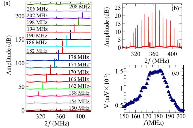
Fig. 3. (a) Voltage spectra for various input RF frequencies in the range of 150–208 MHz. Here, the spectrum was measured every 4 MHz, and each spectrum was vertically shifted to clarify. (b) Voltage spectra for various input RF frequencies signals without offset. (c) Frequency dependence of the dc voltage measured by the previously developed lock-in technique under a small in-plane magnetic field.
