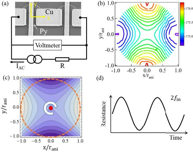
Fig. 1. (a) Scanning electron microscopy image of a part of the fabricated device together with the probe configuration for AMR measurement. (b) Resistance of the circular disks as a function of the vortex core position. (c) and (d) Schematic of the second-harmonic signal generation due to the circular core oscillation.
